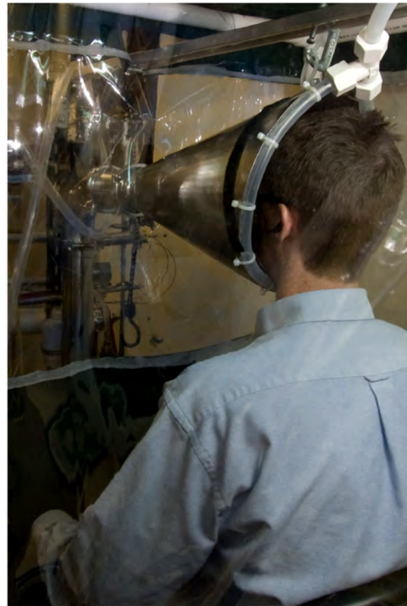
Figure 2. Exhaled breath collection system. Each volunteer sat as shown with face inside the inlet cone of the human exhaled breath air sampler inside a booth supplied with HEPA filtered, humidified air for 30 min while wearing an ear-loop surgical mask. Three times during the 30 min each subject was asked to cough 10 times. After investigators changed the collection media, the volunteer sat in the cone again, without wearing a surgical mask, for another 30 min with coughing as before.
